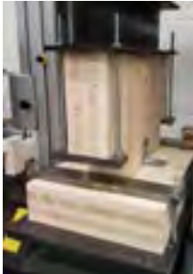
Figure 6: Testing of bracket connection in tension
