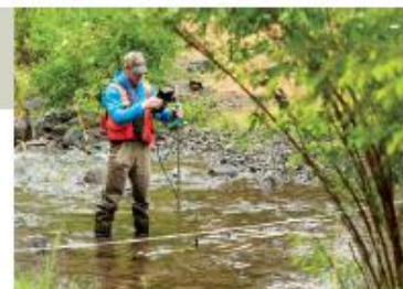
Photo of a field staff taking a flow measurement to help determine the temperature benefit of the restored flow.
